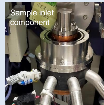
Sample cell for measurement in special environments to evaluate green porous materials
