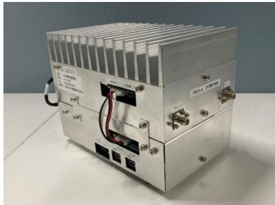
Figure 2: Wireless equipment for the VHF band (220 MHz band) narrowband IoT wireless system
