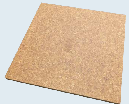
Sustainable building material made from corn and grain stalks
